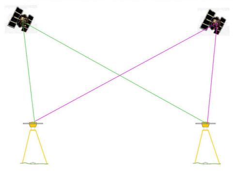
Double differencing: two receivers, two satellites, same epoch (two Single Differences). Eliminates receiver clock error, receiver hardware error, reduces other errors.
