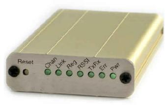
Diagram II-4: CDMA Modem Front Panel (Courtesy of AirLink Comm.)
