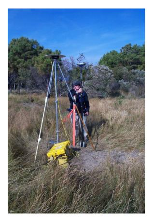
Diagram II-1. The base station should use a ground plane, choke ring, or a current high quality, geodetic, multipath rejecting antenna while the rover typically operates with a smaller antenna (usually integrated with the rover receiver) for ease of use.
