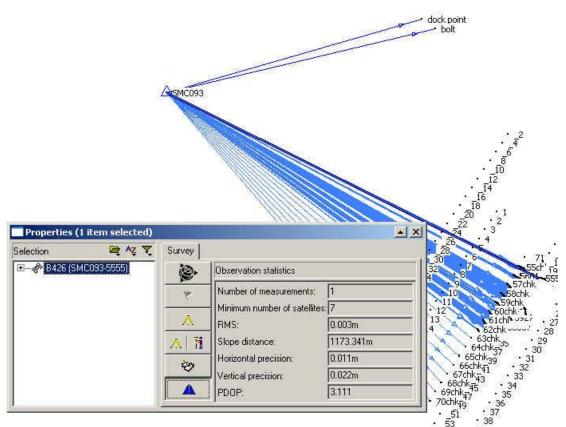
Diagram VI-1. Viewing baseline properties in the GNSS software
