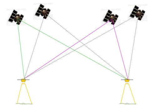
If the receiver retains lock between epochs, the double difference ambiguity remains the same for each epoch and therefore will cancel out in the triple difference equation. If the receiver loses lock, the triple difference solution that contains that loss of lock will show as an outlier and therefore will show the cycle slip during processing.
