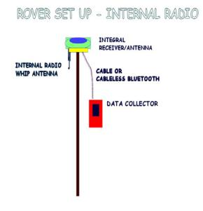
Diagram II-3: Typical UHF Radio Rover Set Up (Receive-Only)
